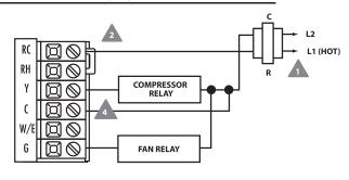
**NOTE:** In many heat pump systems with no emergency heat relay a jumper can be installed between E and W2.
