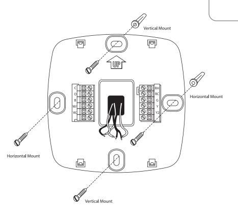
For vertical mount put one screw on top and one screw on bottom.
