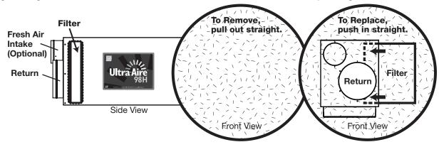
Step 3: Insert filter door into tabs and swing door closed to lock the latch into place.
