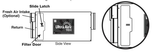
**Step 2:** Remove the filter by gently pulling it straight out of the unit. Insert new filter by gently pushing it straight into the unit. Make sure the AIR FLOW arrow on the filter is pointing into the unit.
