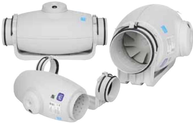
As the name suggests these fans are extremely quiet, low profile "Mixed-flow" fans. Manufactured in plastic material with an external connection box, the body is easily dismantled with a two speed controllable 115V 60Hz motor. Sound waves are directed through the perforated inner skin and absorbed by a layer of sound-absorbent insulation. Plus the TD-SILENT is fitted with rubber gaskets on the inlet and outlet to absorb vibrations.
