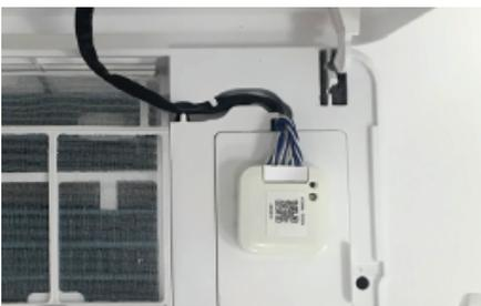
After connecting the air conditioner to the power, the blue LED on the Sensibo Inside device will start blinking.
