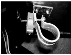
porcelain end-cap (with the 4 pins) through clamp bracket. Be sure to notice the Tension Lever is down.
