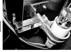
Once the Lamp's end-cap is in place, pull the Tension Lever UP to lock the Lamp in place. If the Lever is loose, just turn Lever clockwise a turn or so. Close and tighten the UV Lamp Access Door.
