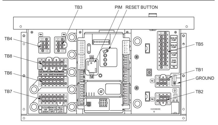
Figure 31. - Control Panel Layout
