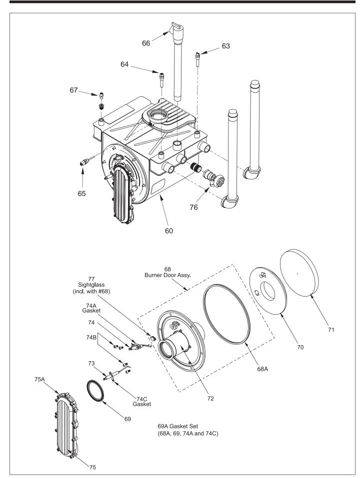
Figure 43. - Heat Exchanger Components
