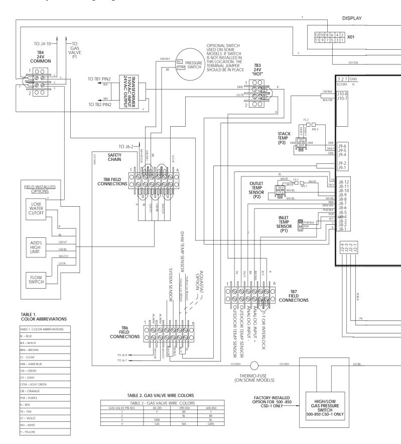
Figure 18. - Wiring Diagram, All Sizes
