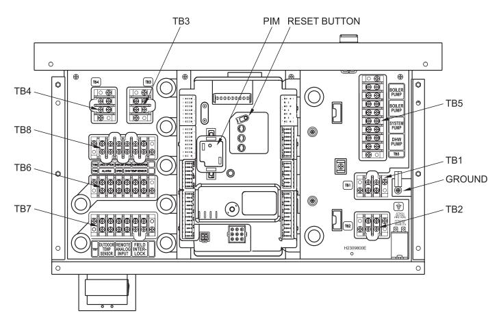
Figure 16. - Control Panel Layout
