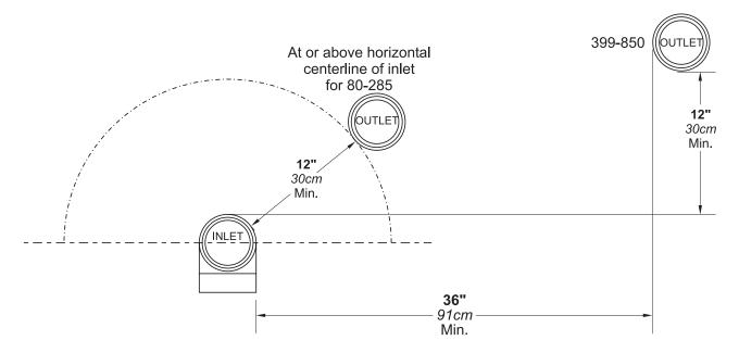
Figure 7. - Minimum Venting Distance
