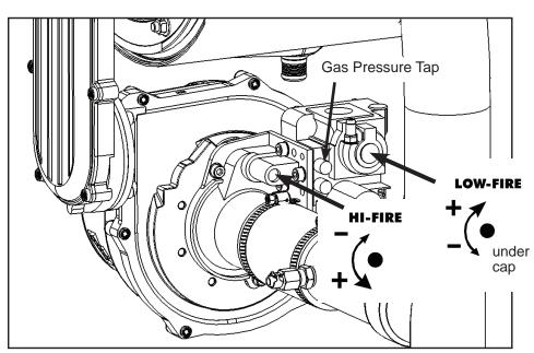
Figure 36. - NeoTherm Gas Valve 80 - 210 Mbtu
