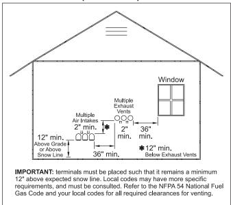
Figure 8. - Multiple Side-Wall Terminals, Air and Vent
