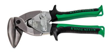
Klein Tools' Upright Snips cut straight, curves, and tight circles in 24 gauge cold rolled steel and 28 gauge stainless steel. This tool makes cutting easier in confined spaces (in ductwork, reaching through openings or against a wall). Soft touch aviation grips provide maximum control and comfort. The blades are made of long-lasting serrated forged steel for superior strength and durability. Tip-Ident® on the handles and color-coding allow for easy identification of the cutting pattern.
