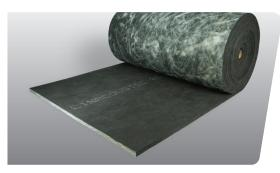
Linacoustic<sup>®</sup> RC insulation is a flexible, fiberglass duct liner. The airstream surface is protected with JM's exclusive reinforced coating system, a glass mat surface coated with Permacote<sup>®</sup> antimicrobial coating.
