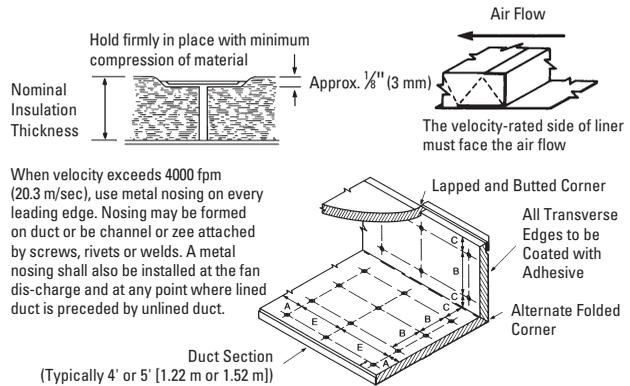
When velocity exceeds 4000 fpm (20.3 m/sec), use metal nosing on every leading edge. Nosing may be formed on duct or be channel or zee attached by screws, rivets or welds. A metal nosing shall also be installed at the fan discharge and at any point where lined duct is preceded by unlined duct.
