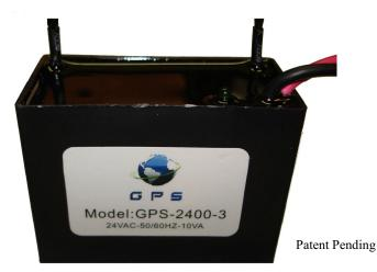
**Product Description:** The GPS-2400 series of products are designed to be mounted inside of fan coils, heatpumps and air handlers up to 2,400 CFM or 6 tons. Their compact size and single screw mounting requirement allows them to be mounted almost anywhere in just a few minutes. The cold plasma produced will travel down the duct disinfecting everywhere the air is traveling.
