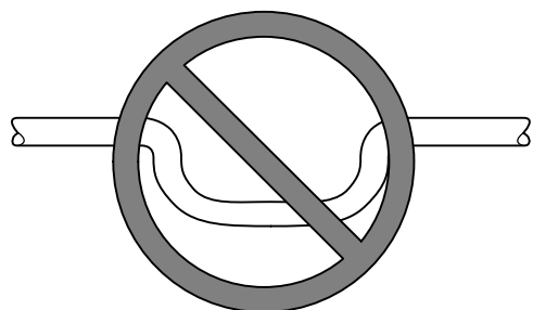
Figure 16 Insufficient Condensate Trap
