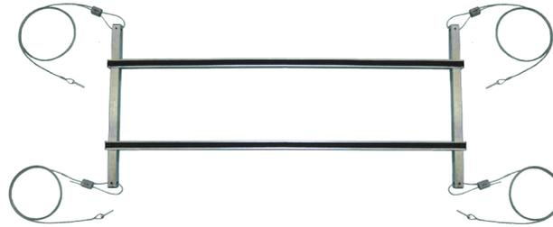
Our hanger utilizes cable locks for quick levelling, and is equipped with a 3<sup>1/2</sup> in. bolt for suspension in a variety of places. Hung-Rite's Hanger gives proper support to eliminate equipment buckling and leaves equipment unobstructed for future maintenance. Pre-drilled holes are located on the arms, for threaded rod during your commercial installations. All of which is available fully assembled in a slender packaging, and ready for your use!
