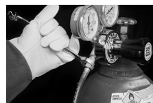
Figure 4. Attaching Hose to Regulator
