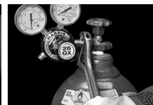
Figure 2. Attaching Oxygen Regulator
