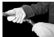
Figure 5. Attaching Hose to Torch
