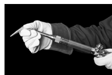
Figure 6. Installing Welding Tip
