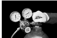
Figure 10. Opening Oxygen valve
