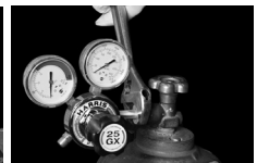
Figure 3. Attaching Fuel Gas Regulator
