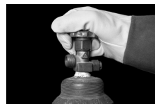
Figure 1. Opening Oxygen Cylinder Valve
