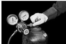
Figure 9. Opening Fuel Gas Cylinder Valve
