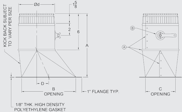
A. HETOs now come standard with sealed joints! The riveted seam on the collar and boot, as well as the co-latch seam between the collar and boot are sealed with the GreenSeam integral gasket. Unsealed fittings are available upon request.
