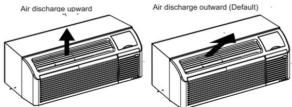
Fig. 16 – Adjusting Louvers
