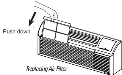
**Fig. 27 – Removing and Replacing Air Filter**
