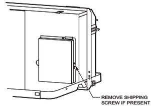
Fig. 13 – Shipping Screw Removal
