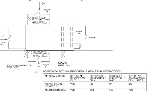
Fig. 21 - Horizontal Return Air Configurations and Restrictions
