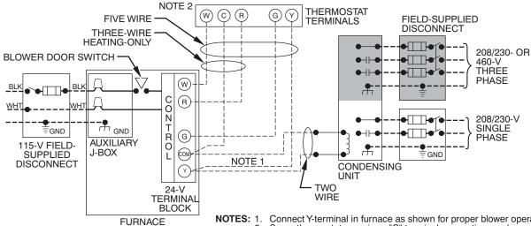
Connect Y-terminal in furnace as shown for proper blower operation. Some thermostats require a "C" terminal connection as shown.
