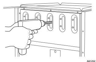
Fig. 47 - Cleaning Heat Exchanger Cell
