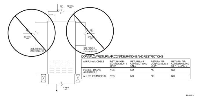
Fig. 20 - Downflow Return Air Configurations and Restrictions
