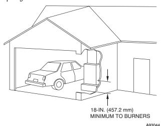
Fig. 5 - Installation in a Garage
