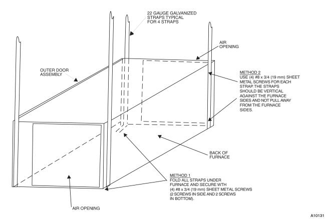
Fig. 16 - Horizontal Suspension with Straps
