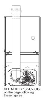
Fig. 31 - Downflow Application-Vent Elbow Up
