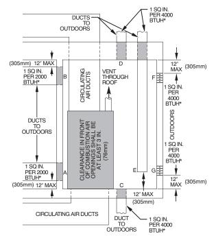
\*Minimum dimensions of 3 in. (76 mm).
