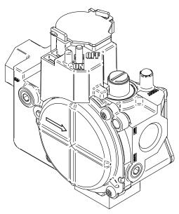
Fig. 41 - Gas Control Valve
