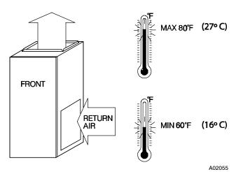
Fig. 3 - Return Air Temperature
