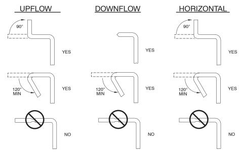
Fig. 14 - Duct Flanges
