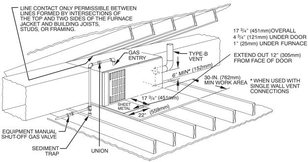
Fig. 17 - Typical Attic Installation
