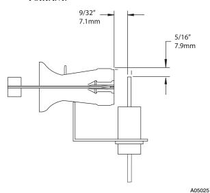
Fig. 45 - Igniter Position-Side View
