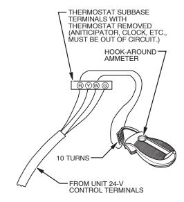
EXAMPLE:  $\frac{5.0 \text{ AMPS ON AMMETER}}{10 \text{ TURNS AROUND JAWS}} = \frac{0.5 \text{ AMPS FOR THERMOSTAT}}{\text{ANTICIPATOR SETTING}}$
