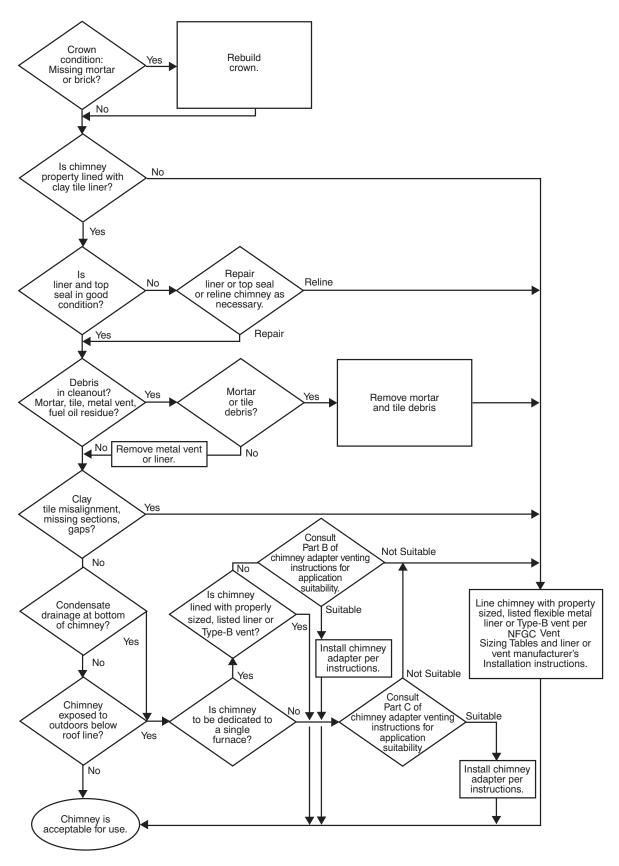
Fig. 27 - Chimney Inspection Chart
