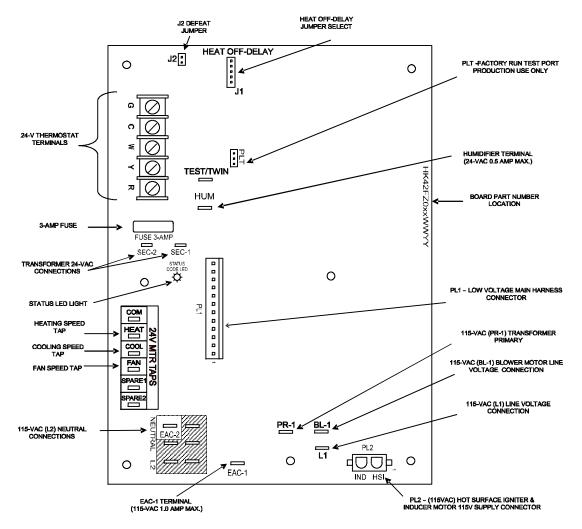
Fig. 24 - Furnace Control
