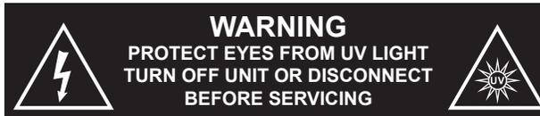
**Important:** some materials inside the air system (including filter media, flex duct, wiring etc.) may not be UV light resistant. Use the optional UV shield (part #TUV-SHIELD-LPC) or cover the materials with reflective tape.
