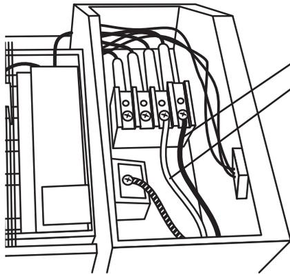
1. Remove the control box cover and connect the wiring harness as shown.
