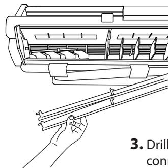
2b. For systems with non-removable drain pan, remove louvers and baffles to access the area behind.
