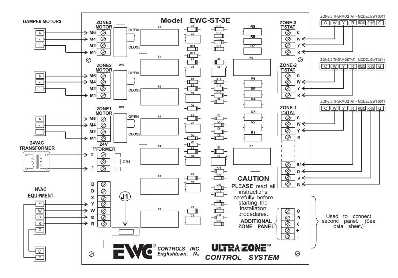
All wiring should be done to local and national codes and ordinances. Use color-coded multi-conductor wire. Wire number to number or letter to letter on each control.
