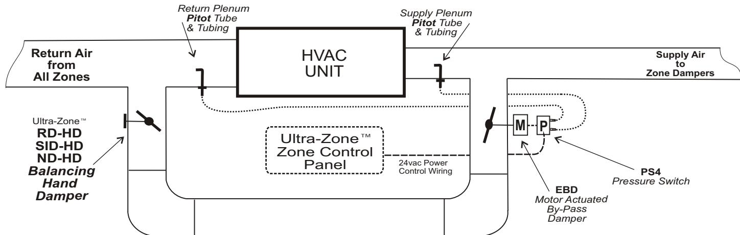
Note: This drawing of the bypass damper static pressure control and related duct work is intended to serve as a guide. Your actual duct configuration may differ and that's OK, so long as all components are installed correctly.
