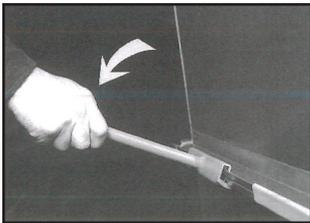
17. WDCI cleat can be snapped-on with the Cleater I Tool or with the Cleater II where space is restricted.
