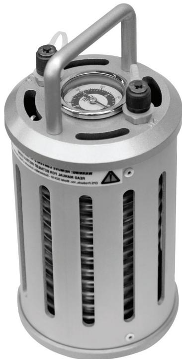
The effects of ambient temperature and elevated tank pressures on the speed of the refrigerant recovery process are in many cases more important than the speed of the recovery machine itself. As the ambient temperature increases, the pressure in the recovery cylinder increases, significantly reducing the recovery speed and in many cases can lead to a high pressure shutdown as the recovery equipment and tank pressure limits are reached.
