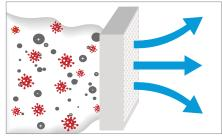
Captured airborne microbes remain on the pleated filter instead of recirculating back into the home and are subjected to an intense electric field.
