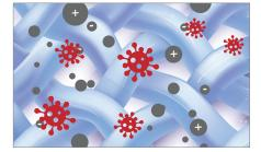
The ionized particles are pulled toward an oppositely charged, pleated filter and captured at an extremely high rate, similar to how a magnet attracts metal shavings.
