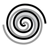
As the spiral continues to orbit, the gas is compressed into two increasingly smaller pockets.
