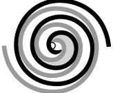
By the time the gas arrives at the center port, discharge pressure has been reached.
