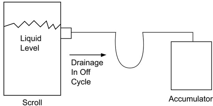
To prevent flooded start damage due to off cycle migration, the accumulator may be configured on some systems to allow free drainage from the compressor to the accumulator during the off cycle. When the above configuration is not possible and the unit charge is over the charge limit shown in Table 5, a crankcase heater is required.
