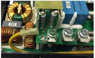
4. There are (5) screws attaching the fuse board on the inverter (2) – T20 and (3) – T10 Torx. After removing these screws the fuse board can be removed and replaced.
