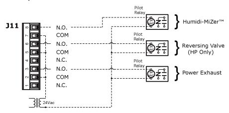
NOTE Output relay contacts rated at 3A, 24V maximum. Install pilot relays required by application.
