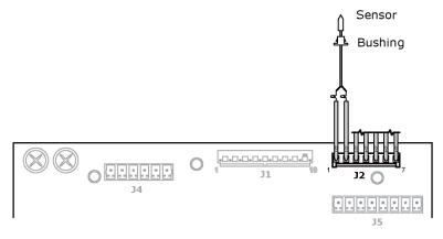
NOTE Sensor termination requires installation of RTU Open wiring harness assembly (Part #OPN-RTUHRN).
