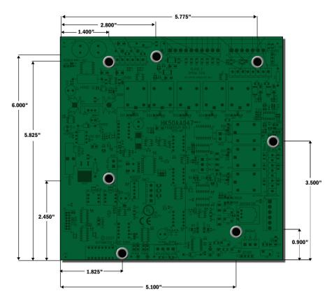
RTU Open v3 Installation and Start-up Guide Carrier Proprietary and Confidential
