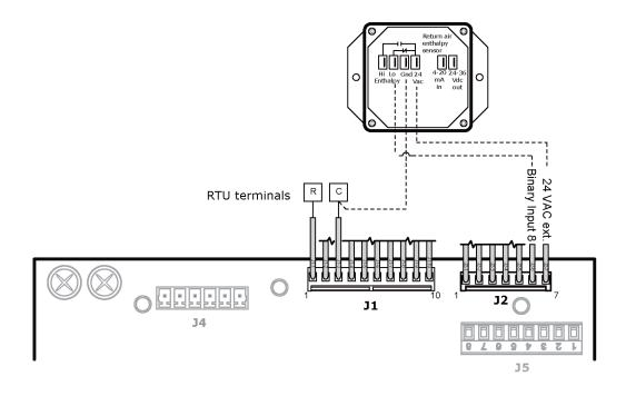
NOTE Factory-installed enthalpy switches terminate at J2 wires 6 (switch input) and 7 (24 Vac).
