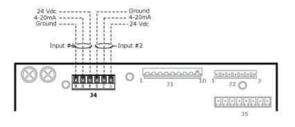
**NOTE J4** Analog Inputs 1 and 2 may be set for the following device types:
