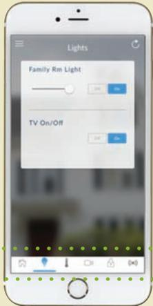
Press the Lights icon
