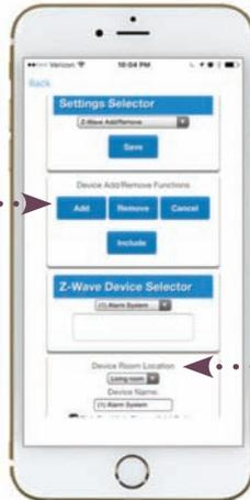
**Step 3.** Once learned, place the Z-Wave device in desired location and designate the location of the Z-Wave device by selecting the **Device Room Location** from the drop down menu.
