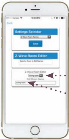
Select Z-Wave Room Names from the drop down menu to modify the display name of the referenced room where a Z-Wave component will be used.
