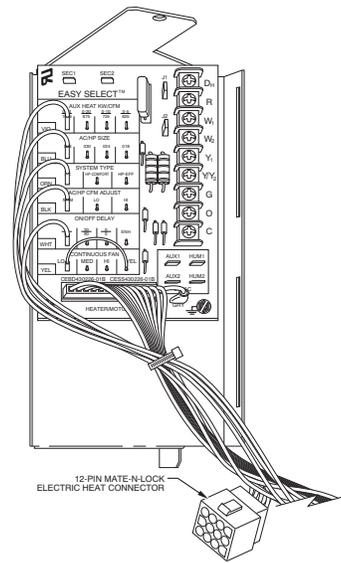
**Fig. 18 - Detail of FV4C Printed-Circuit Board**
