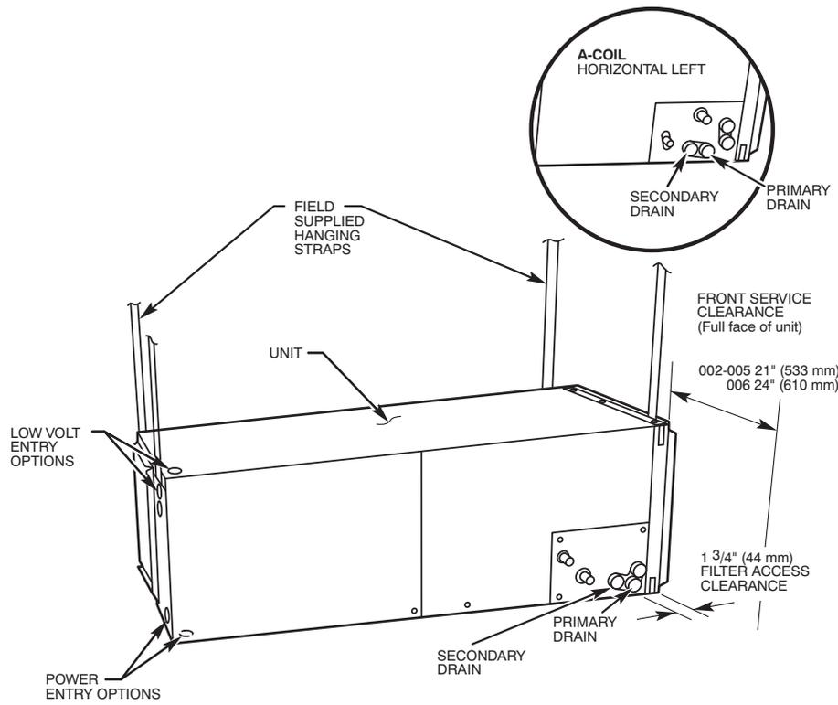
**Fig. 3 - Slope Coil in Horizontal-Left Application (Factory Ready)**
