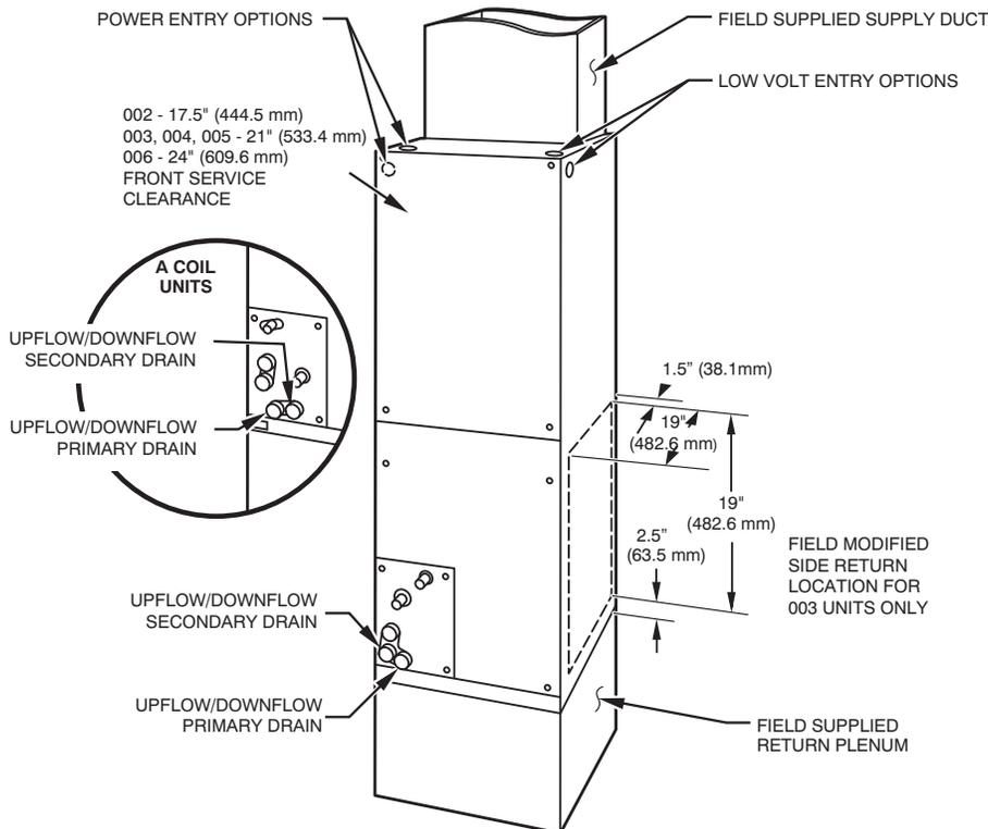
Fig. 2 - Slope Coil Unit in Upflow Application
