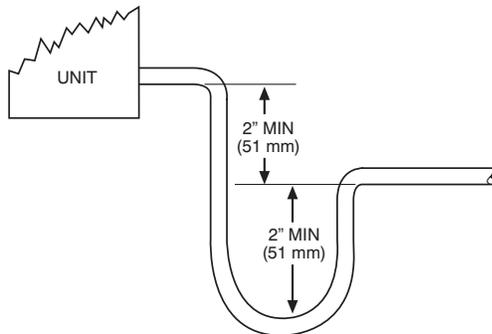
Fig. 14 - Recommended Condensate Trap
