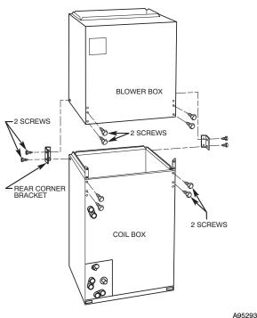
Fig. 5 - Modular Unit Assembly
