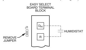
Fig. 20 - Humidistat Wiring for De-Humidify Mode
