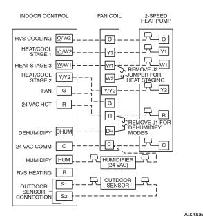
Fig. 12 - FV4C Fan Coil Wiring with 2-Speed Puron (R-410A) Refrigerant Heat Pump
