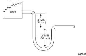
Fig. 14 - Recommended Condensate Trap
