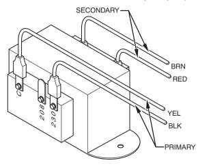
Fig. 13 - Transformer Connections
