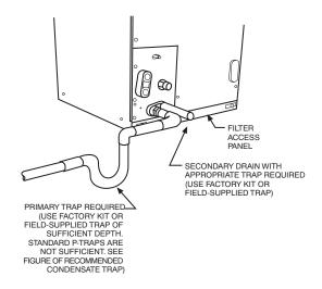
Fig. 16 - Insufficient Condensate Trap
