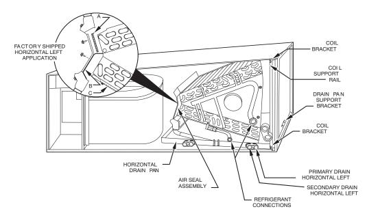
Fig. 4 - A-Coil in Horizontal-Left Application (Factory Ready)
