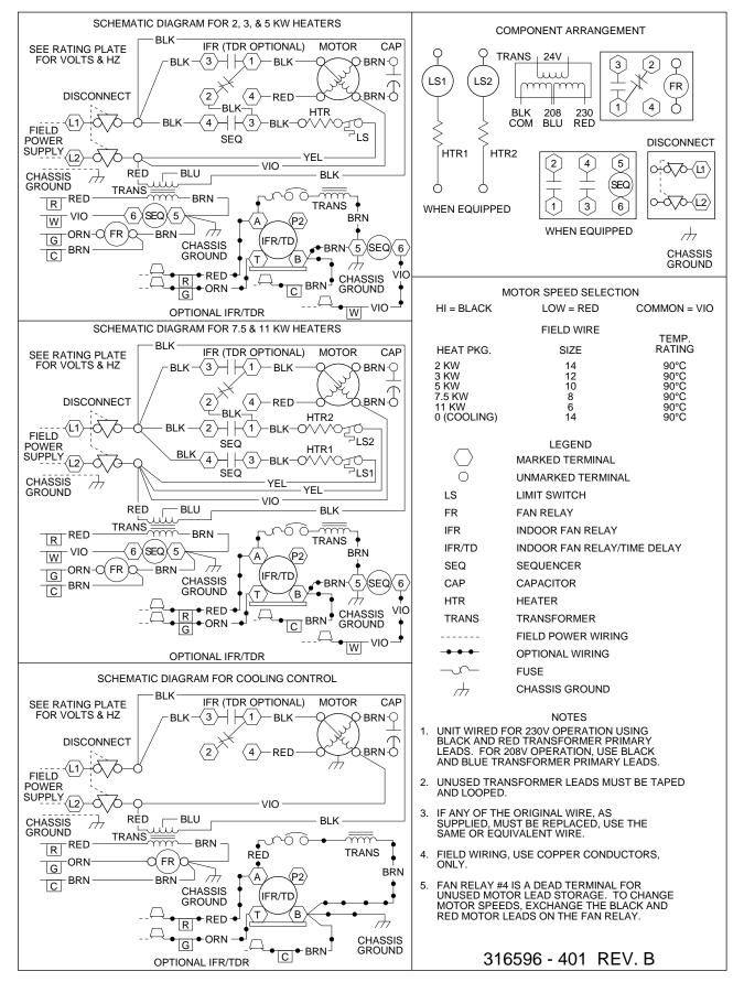
Fig. 33—FF1A/FF1B/FF1C Typical Unit Wiring Label
