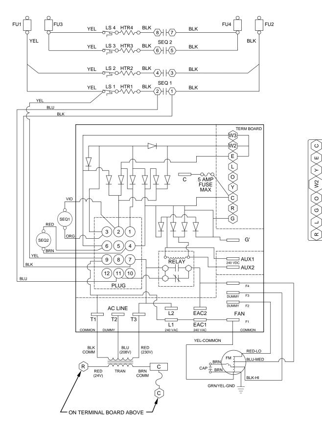
Fig. 13—Wiring Schematic
