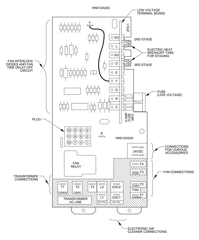
Fig. 7—HK61GA003 Printed-Circuit Board
