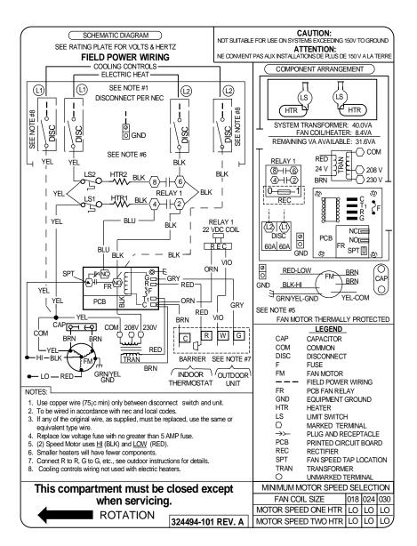
Fig. 3B—FF1D Typical Wiring Diagram
