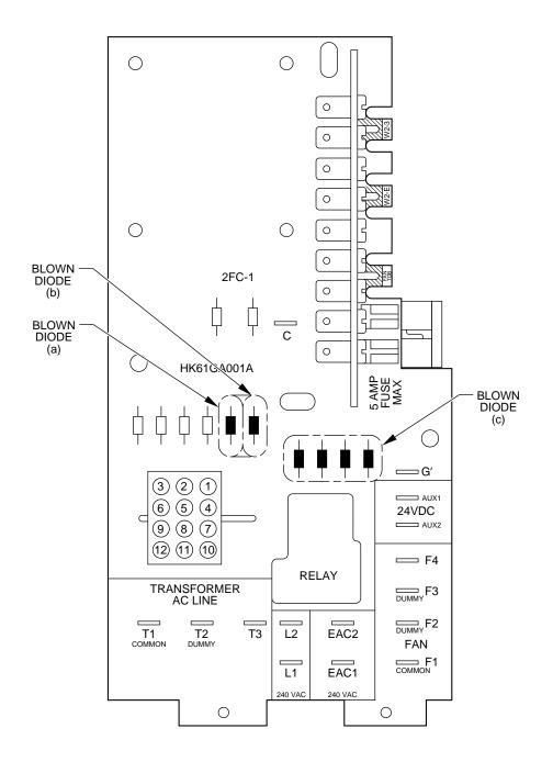
Fig. 14—Control Board Noting Diodes
