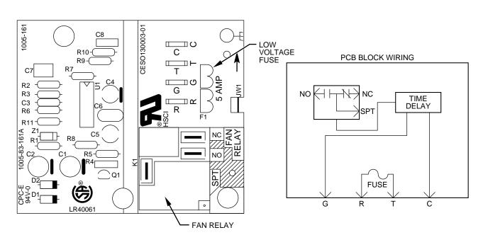
Fig. 3A—Fan Coil Printed-Circuit Board
