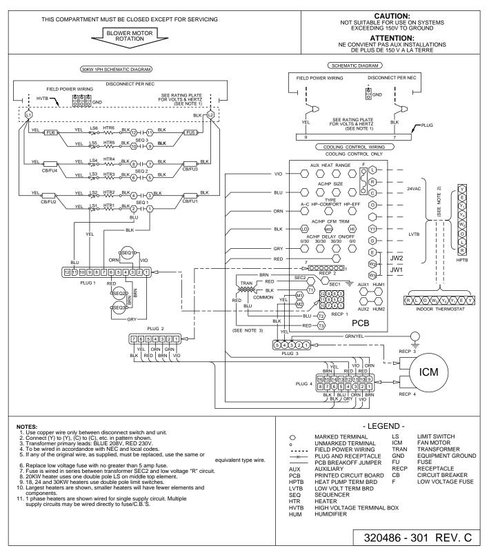
3. Check power leads L1 and L2. If these are not receiving power, system cannot function.
