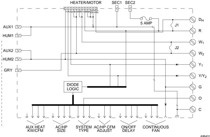
Fig. 25—Easy Select Board Schematic
