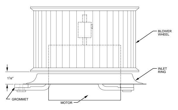
Fig. 34—FF1A/FF1B/FF1C Motor, Inlet Ring, and Blower Wheel Assembly
