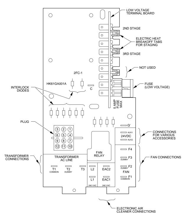
Fig. 6—HK61GA001 Printed-Circuit Board
