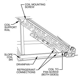
Fig. 32—Slope Coil Component Location
