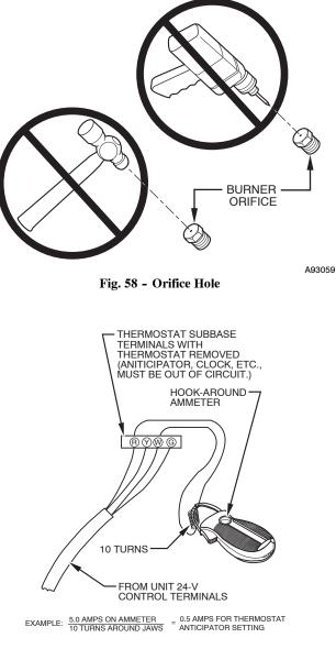
Fig. 59 - Amp. Draw Check with Ammeter
