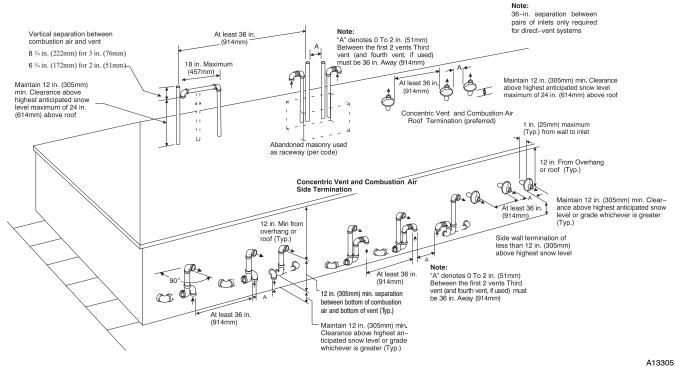
Fig. 51 - Combustion Air and Vent Pipe Termination for Direct Vent (2-Pipe) System
