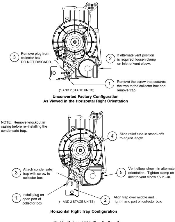
Fig. 10 - Horizontal Right Trap Configuration (Appearance may vary) A11573
