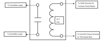
Fig. 34 - Field-supplied Isolation Relay for Humidifiers with Internal Power Supply
