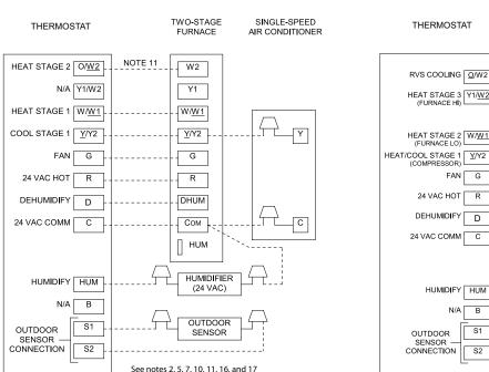
Modulating and 2-Stage Furnace with Single-Speed Air Conditioner
