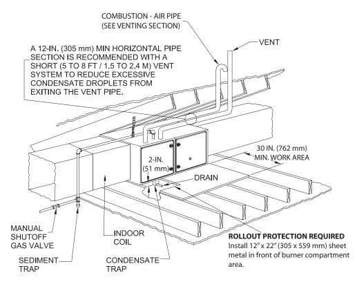
NOTE: FURNACE SHOWN AS DIRECT VENT APPLICATION. REFER TO THE VENTING SECTION FOR ALLOWABLE VENT CONFIGURATIONS
