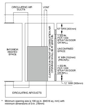
† Minimum of 3-in. (76mm) when type-B1 vent is used.
