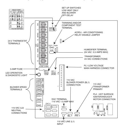
Fig. 36 - Example of Two-Stage Furnace Control
