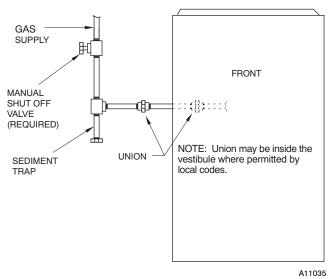
Fig. 31 - Typical Gas Pipe Arrangement
