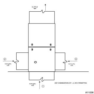
Fig. 25 - Upflow Return Air Configurations and Restrictions
