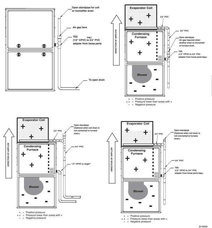
Fig. 14 - Example of Field Drain Attachment
