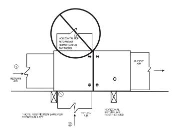
Fig. 27 - Horizontal Return Air Configurations and Restrictions
