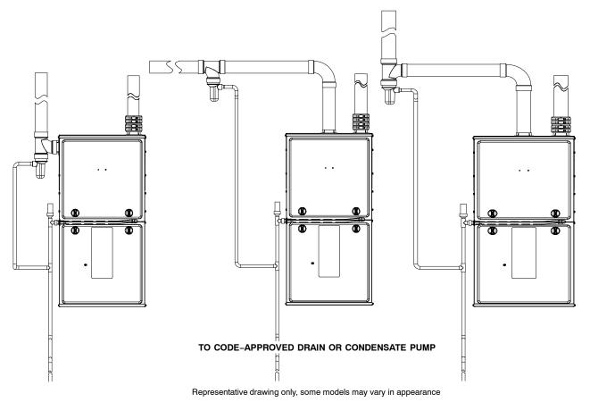
Fig. 56 - Recommended Combustion Air Inlet Moisture Trap
