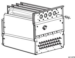
Fig. 65 - Cleaning Heat Exchanger Cell
