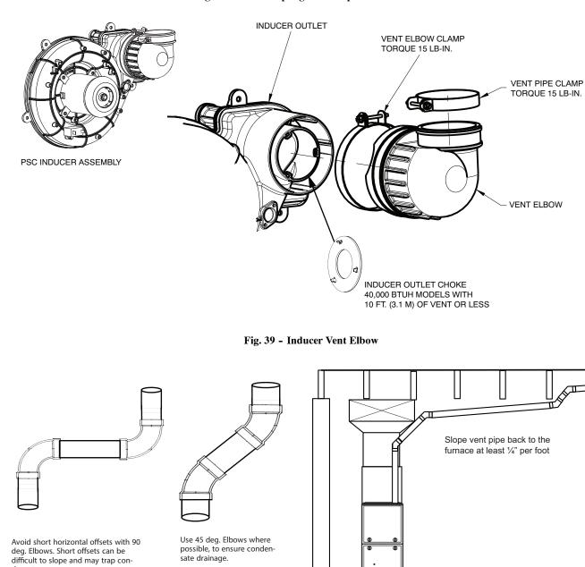
Fig. 40 - Near Furnace Vent Connections
