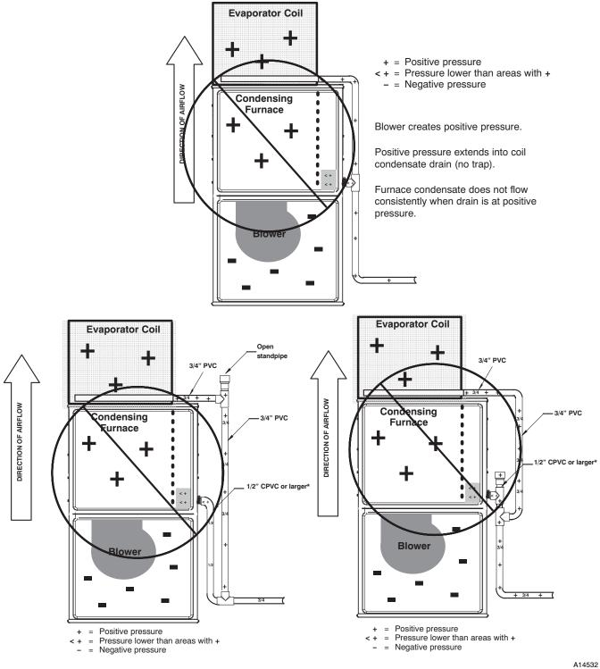
Fig. 13 - Example of Field Drain Attachment (Not Allowed)
