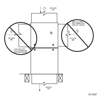
Fig. 26 - Downflow Return Air Configurations and Restrictions
