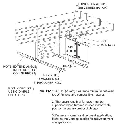
Fig. 29 - Suspended Furnace Installation
