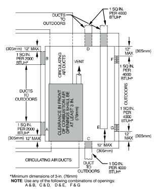
Fig. 6 - Air for Combustion, Ventilation, and Dilution for
