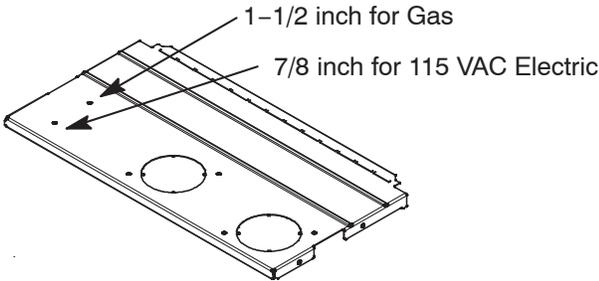
**Fig. 33 – Alternate Gas and Electric Entry**
