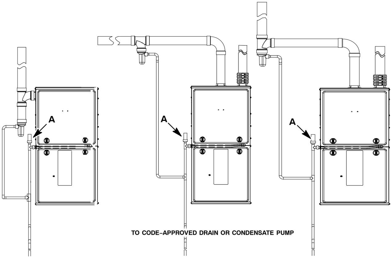
Recommend "T" fitting with 4-inch minimum height standpipe (A) of same diameter or larger extending upward.
