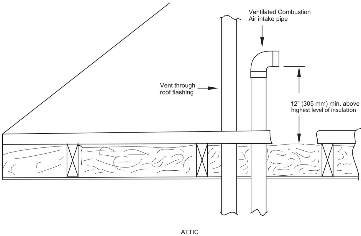
Fig. 56 – Vent Terminations for Ventilated Combustion Air
