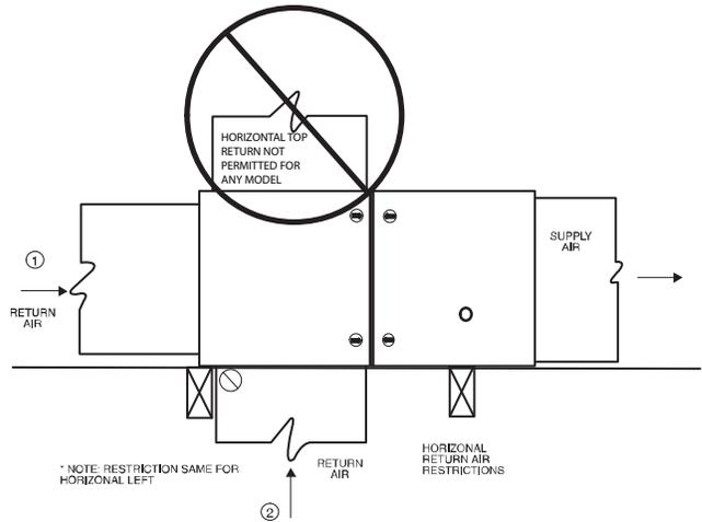
**Fig. 29 - Horizontal Return Air Configurations and Restrictions**
