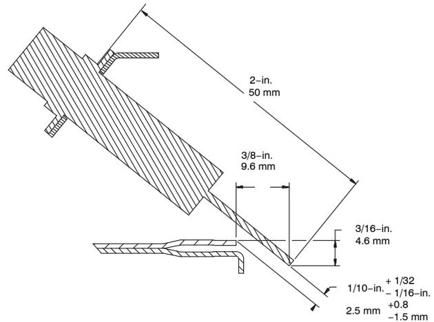
Fig. 64 - Igniter Position - Side View
