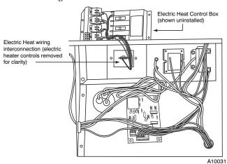
Fig. 11 - Control Box Wiring
