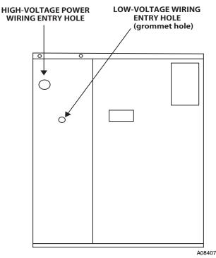
Fig. 10 - Unit Electrical Connection
