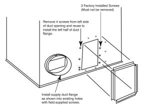
X = Factory dimples for duct flange attachment.
