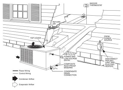
Fig. 7 - Typical Installation
