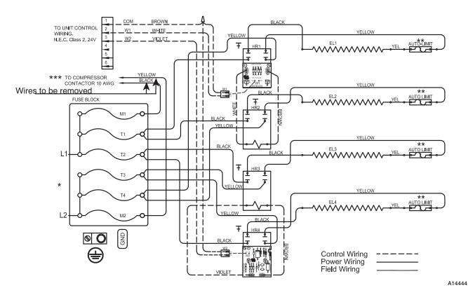
Fig. 15 - Accessory Electric Heater Wiring
