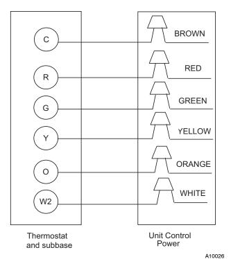
Fig. 13 - Control Connections
