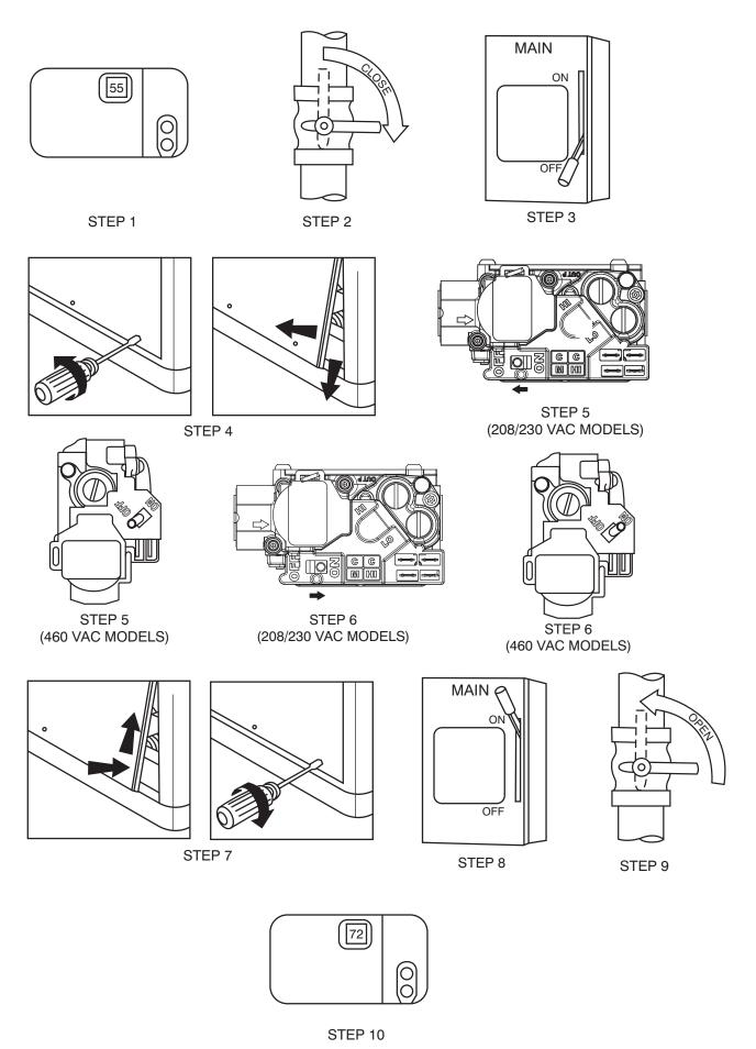
Fig. 4 - To Start Unit Gas Heat
