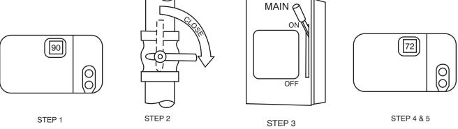
Fig. 6 - To Start Unit Electric Cooling
