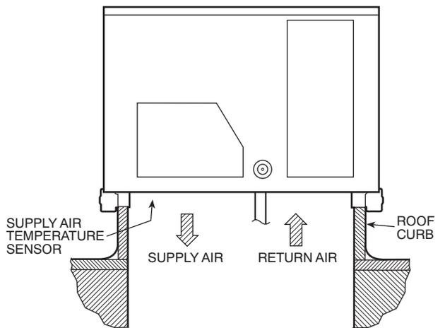
**Fig. 43 - Typical Mounting Location for Supply Air Temperature (SAT) Sensor on Small Rooftop Units**
