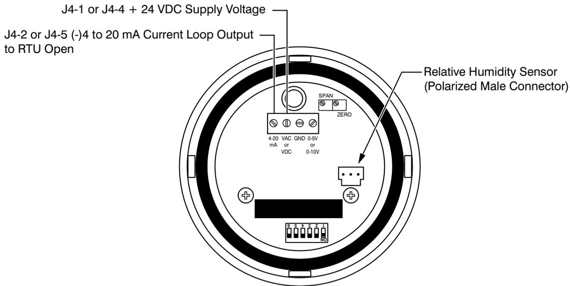
**Fig. 69 - Duct Relative Humidity Sensor Typical Wiring**
