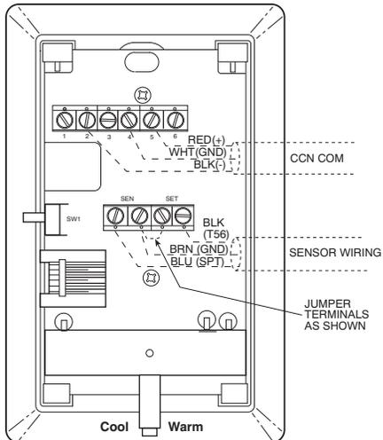
**Fig. 46 - T-56 Internal Connections**
