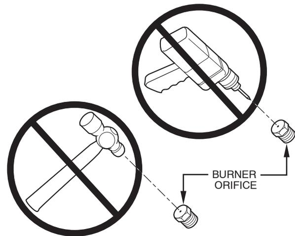
**Fig. 21 - Orifice Hole**
