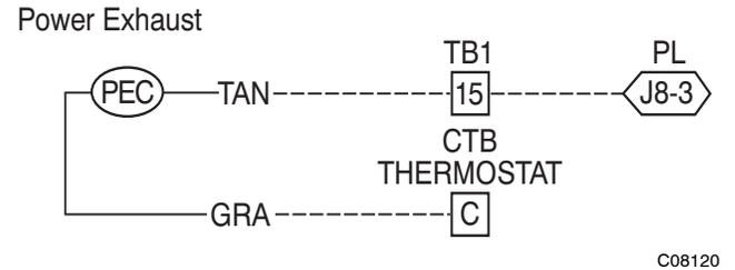
**Fig. 58 - PremierLink Power Exhaust Output Connection**
