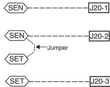
**Fig. 64 - RTU Open T-56 Sensor Connections**
