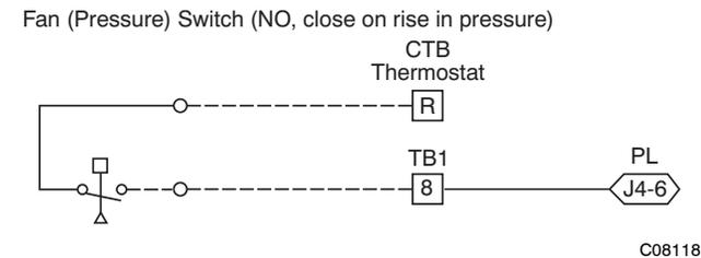
**Fig. 56 - PremierLink Wiring Fan Pressure Switch Connection**
