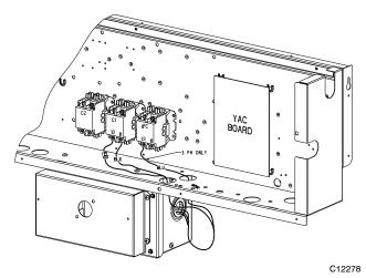
Fig. 26 - Location of Non-Fused Disconnect Enclosure
