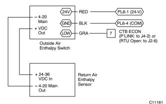
Fig. 75 - Outside and Return Air Enthalpy Sensor Wiring
