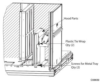
Fig. 9 - Economizer and Two-Position Damper Hood Parts Location
