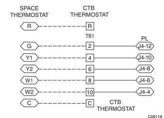
Fig. 48 - Space Thermostat Connections
