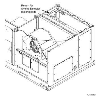
Fig. 76 - Return Air Smoke Detector, Shipping Position
