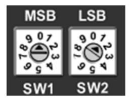
Fig. 71 - RTU Open Address Switches
