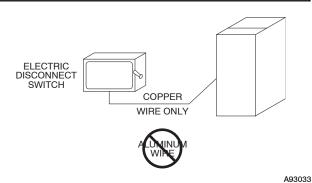
Fig. 25 - Disconnect Switch and Unit
