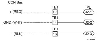
Fig. 59 - PremierLink CCN Bus Connections
