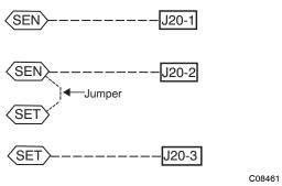
Fig. 64 - RTU Open T-56 Sensor Connections
