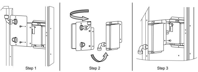
Fig. 77 - Completing Installation of Return Air Smoke Sensor
