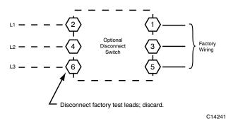
Fig. 24 - Power Wiring Connections
