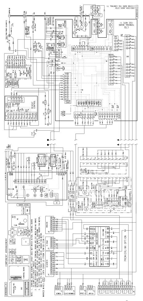
Fig. 42 - PremierLink Wiring Schematic with Humidi-MiZer®
