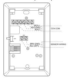
Fig. 44 - T-55 Space Temperature Sensor Wiring
