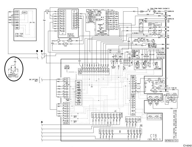
Fig. 36 - Typical Humidi-MiZer® Adaptive Dehumidification System Humidistat Wiring
