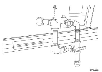
Fig. 20 - Gas Piping Thru-Base Connections
