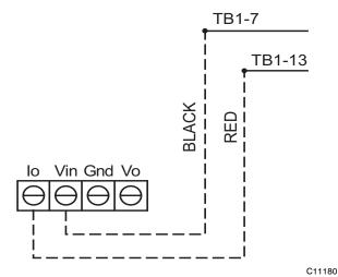
Fig. 54 - Space Relative Humidity Sensor Connection
