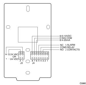
Fig. 49 - Indoor/Outdoor Air Quality (CO<sub>2</sub>) Sensor (33ZCSENCO<sub>2</sub>) - Typical Wiring Diagram
