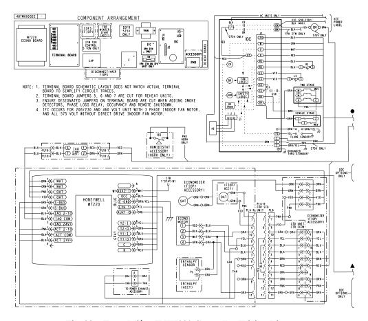
Fig. 38 - EconoMi\$er X W7220 Controller Wiring Diagram
