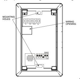
Fig. 53 - Space Relative Humidity Sensor Installation
