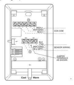
Fig. 46 - T-56 Internal Connections
