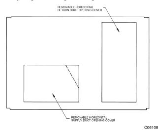
Fig. 7 - Horizontal Conversion Panels
