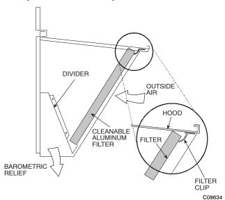
Fig. 12 - Economizer Filter Installation
