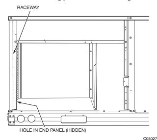
Fig. 33 - Field Control Wiring Raceway
