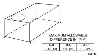
Fig. 4 - Unit Leveling Tolerances
