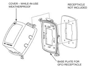
Fig. 29 - Weatherproof Cover Installation
