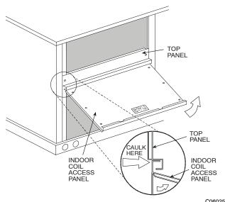
Fig. 10 - Indoor Coil Access Panel Relocation
