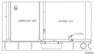
Fig. 13 - Compressor Door Latch Location
