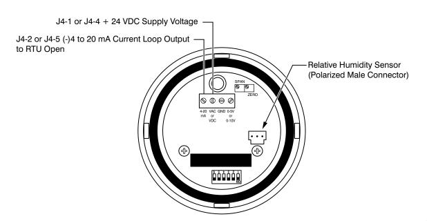
Fig. 69 - Duct Relative Humidity Sensor Typical Wiring
