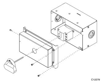
Fig. 27 - Handle and Shaft Assembly for NFD
