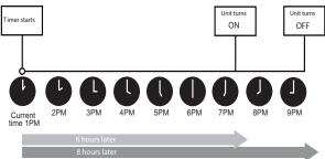
Fig. 16 Set both Timer ON and Timer OFF
