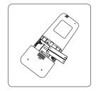
Remove batteries from remote control
