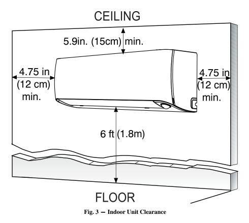
**NOTE**: The top clearance recommended for proper return airflow is 5.9in (15cm). Reduction of this clearance may decrease the performance of these units. This may be reduced to 3.2in (80mm) as long as the right and left clearances are achieved.
