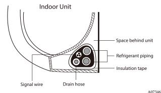
**Fig. 21 — Bundle drain hose, refrigerant pipes, & signal cable NOTE:** For applications where gravity cannot be used for drainage, a condensate pump accessory is available. Consult the condensate pump Installation Instructions for more information.
