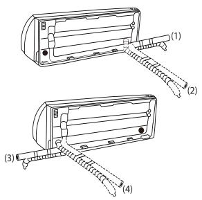
Fig. 8 – Piping Angle
