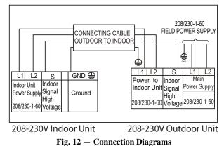
Notes: 1. Do not use thermostat wire for any connection between indoor and outdoor units. 2. All connections between indoor and outdoor units must be as shown. The connections are sensitive to polarity and will result in a fault code.
