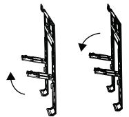
Fig. 10 – Use Holder to Prop up the Unit
