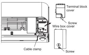
Fig. 13 - Terminal Block Location
