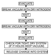
Fig. 22 — Triple Evacuation Method
