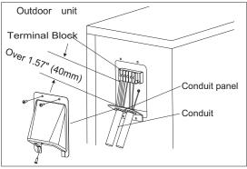
Fig. 13 - Field Wiring
