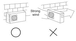
Fig. 11 — High Wind Installation
