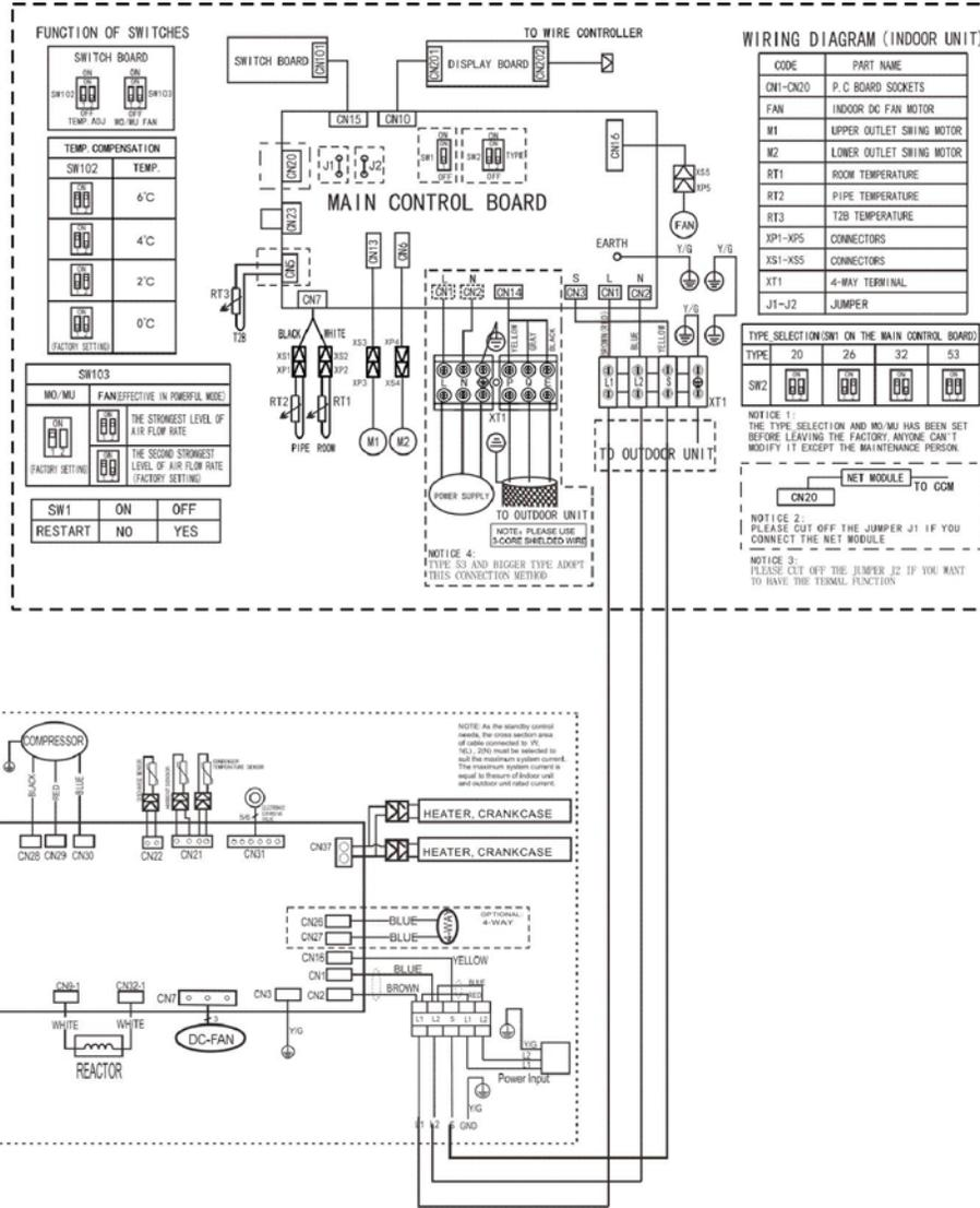
Fig. 7 – Wiring Diagram Sizes 9 and 12
