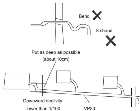
**Fig. 21 – Condensate Flow**
