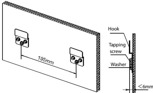
**Fig. 5 – Anchor the hooks**
