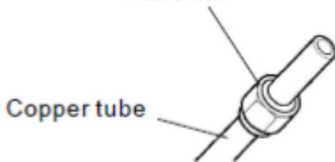
**Fig. 20 – Flare nut and copper tube**
