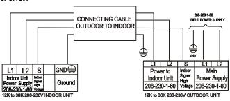
Fig. 26 — Connection Diagrams
