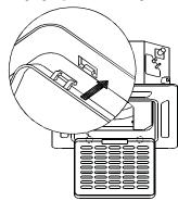
Fig. 21 — Mount the Intake Grille
