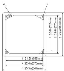
Fig. 4 — Drilling Holes
