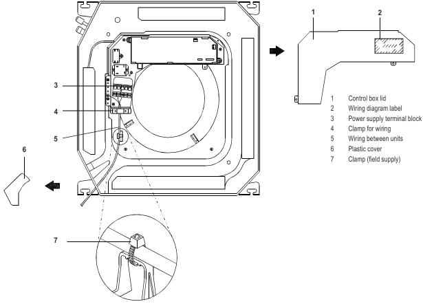
Fig. 16 - Wiring/Control Box
