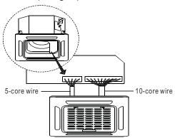
Fig. 22 — Connect the two wires
