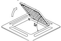
Fig. 18 — Open Intake Grille
