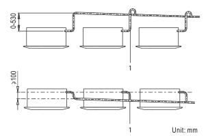
T-joint converging drain pipes
