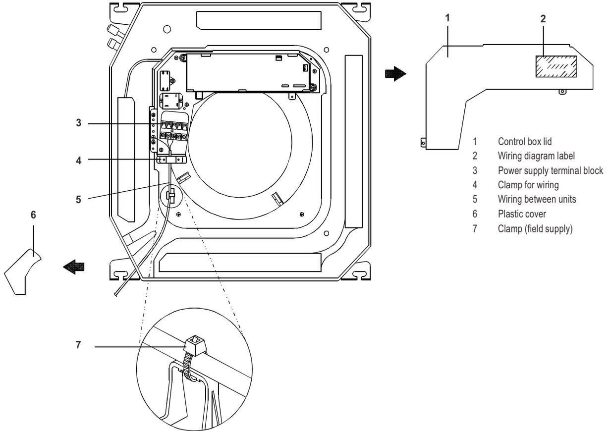
**Fig. 16 – Wiring/Control Box**
