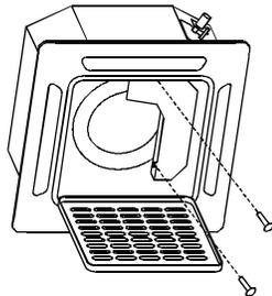
**Fig. 24 – Fasten the Control Box Lid**
