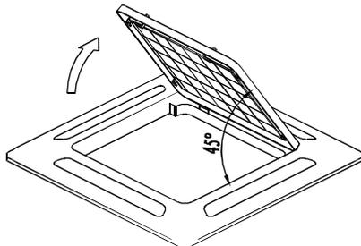
**Fig. 18 – Open Intake Grille**
