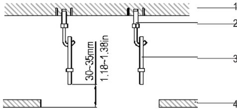
**Fig. 7 – Installation Clearances**
