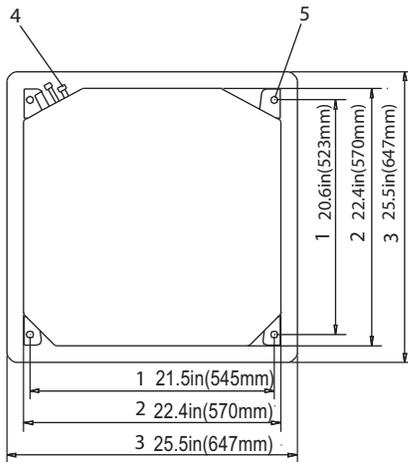
**Fig. 4 – Drilling Holes**
