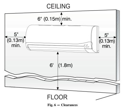
**NOTE**: The top clearance recommended for proper return airflow is 5.9in (15cm). Reduction of this clearance may decrease unit performance. This may be reduced to 3.2in (80mm) as long as the right and left clearances are achieved.
