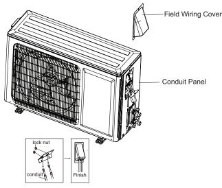
Fig. 16 - Field Wiring
