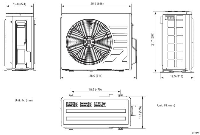
Fig. 3 - 12K 230V (Net Operating Weight: 63.8 lbs. / 30 kg)
