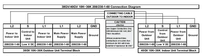
NOTE: Polarity of power wires must match original connection on outdoor unit.
