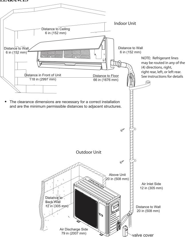
Fig. 6 - Indoor and Outdoor Unit Clearances
