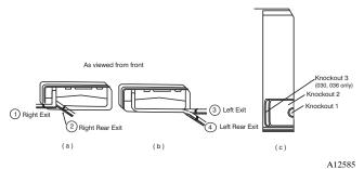
Fig. 12 - Refrigerant Line Routing
