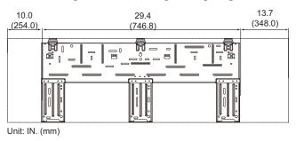
Fig. 10 - 30/36k Mounting Plate Spacing
