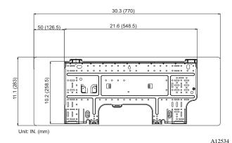
Fig. 7 - 09 and 12K Mounting Plate Spacing
