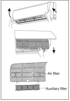
Fig. 25 - Install Air Filter
