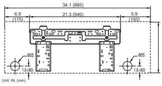
Fig. 8 - 18k Mounting Plate Spacing
