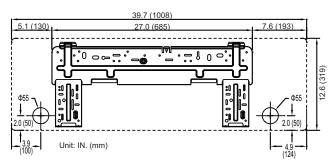
Fig. 9 - 24k Mounting Plate Spacing
