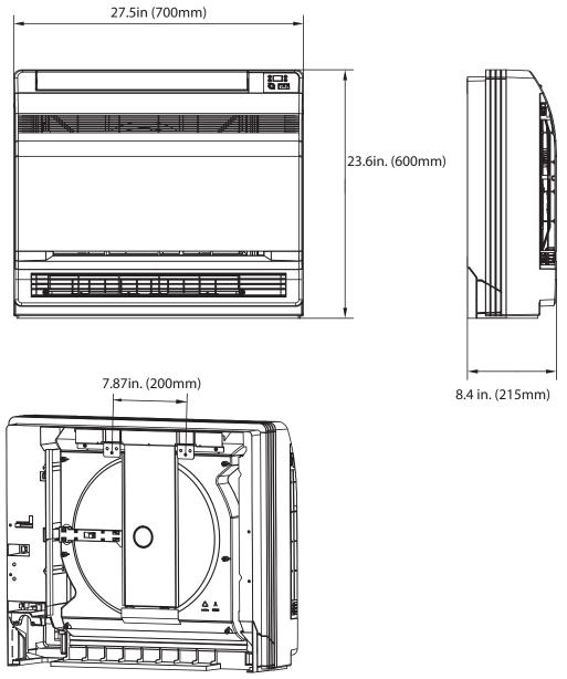
**Fig. 7** – Floor Console Dimensions
