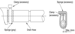
Fig. 58 – Drain Hose Insulation
