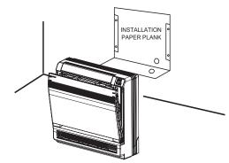
Fig. 63 – Installation Paper Plank
