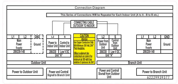
Fig. 84 – Connection Diagram Branch Box
