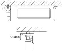
Fig. 48 – Install the indoor unit
