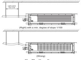
Fig. 57 – Slope Degree
