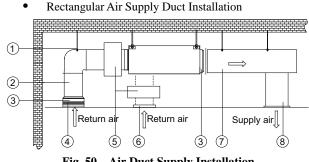
Fig. 50 – Air Duct Supply Installation
