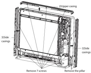
Fig. 71 – Remove the screws
