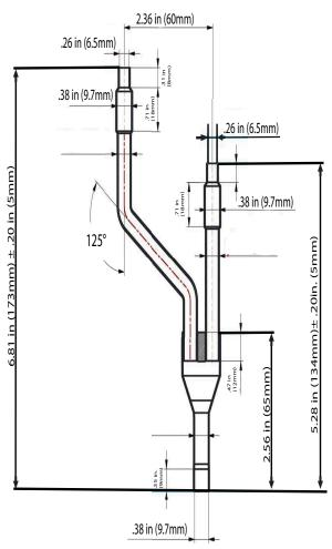
Fig. 21 – Branch Pipe – Liquid Pipe
