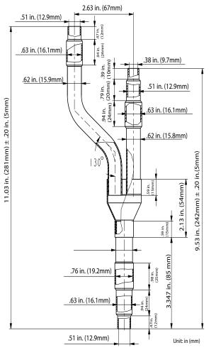
Fig. 20 – Branch Pipe – Gas Pipe
