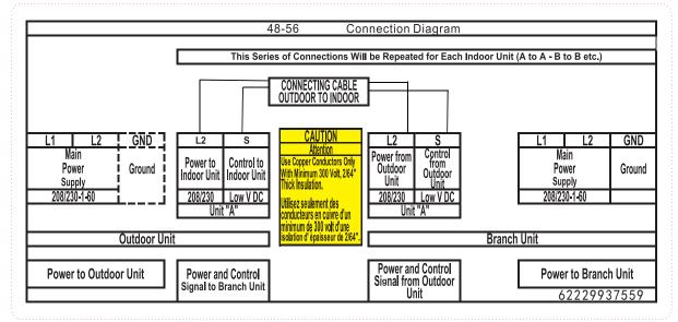
Fig. 83 – Connection Diagram Sizes 48–56
