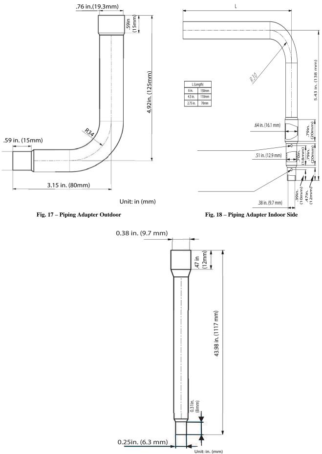
Fig. 19 – Piping Adapter Indoor Side (Liquid)
