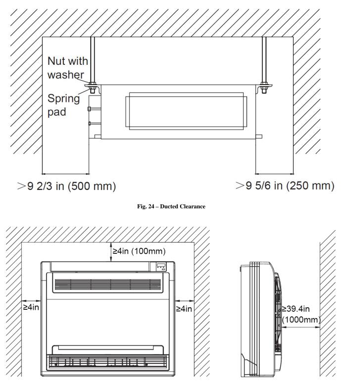
Fig. 25 – Floor Console Clearance
