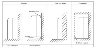
Fig. 61 – Indoor Unit Installation Drawings
