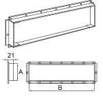
Fig. 52 – Air Supply Outlet
