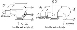
Fig. 55 – Return Air Duct
