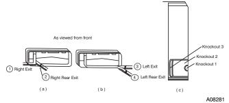
Fig. 28 - Refrigerant Line Routing
