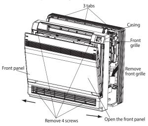
Fig. 70 – Remove the screws
