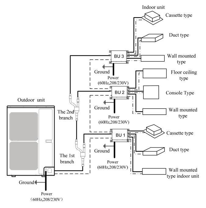
Fig. 79 – Connection Flow
