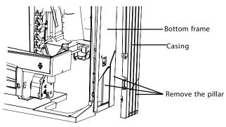
Fig. 73 – Remove the pillar
