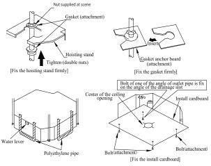
Fig. 33 – Hoisting the main body
