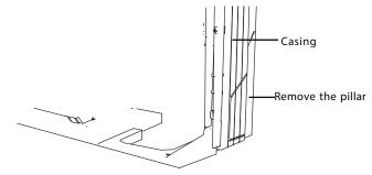
Fig. 72 – Remove the pillar
