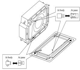
Fig. 45 – Connect Joints
