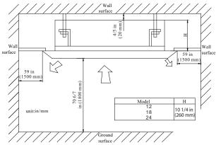
Fig. 30 – Schematic diagram of installation spaces Select install location of the indoor unit
