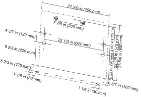
Schematic drawing of hooks:
