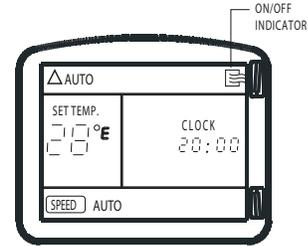
When the air conditioner is not in operation, the remote control will display the last set point, mode and time.
