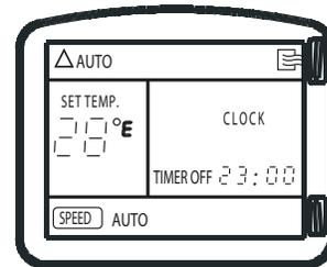
This function will allow the unit to stop automatically at the set time. The timer can be set while the unit is on or while it is off.
