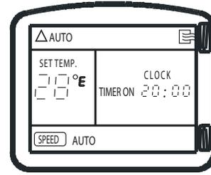
This function will allow the unit to start automatically at the set time. The TIMER ON can be set while the unit is on or off.
