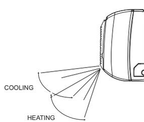
The horizontal louvers can be adjusted using the remote control and can be set to be stationary or moving continuously.
