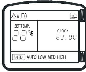
The fan speed can be selected by pressing the **FAN SPEED** button.
