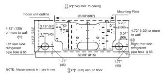
Fig. 5 - Mounting Plate- Model size 009
