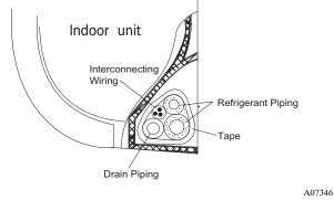
Fig. 16 – Proper Orientation
