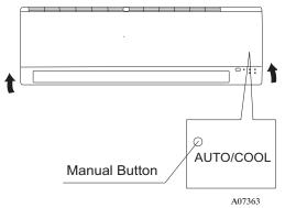
Fig. 22 – Test Operation
