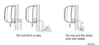
Fig. 15 – Proper Drain Hose Installation
