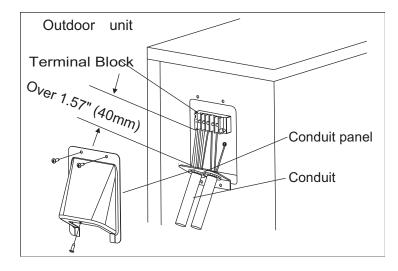
Fig. 12 - Field Wiring
