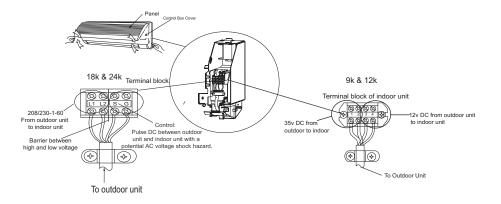
Fig. 17 - Control and Power Wiring on Indoor Unit
