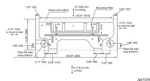
Fig. 6 – Mounting Plate- Model size 012
