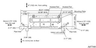
Fig. 7 – Mounting Plate- Model sizes 018 - 024
