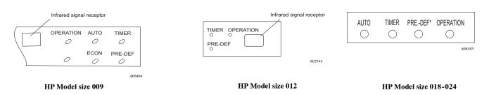
\* PRE-DEF light will illuminate when the unit is running in FAN ONLY mode on Cooling Only units. Note: Cooling only units have same LED lights but without PRE-DEF print.
