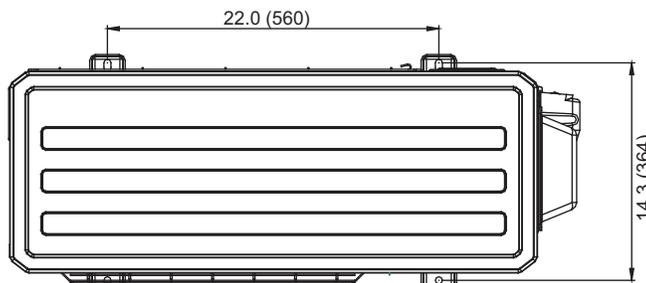
**Fig. 4 – 18K and 24K (Net Operating Weight: 112.2 lbs. / 51 kg)**
