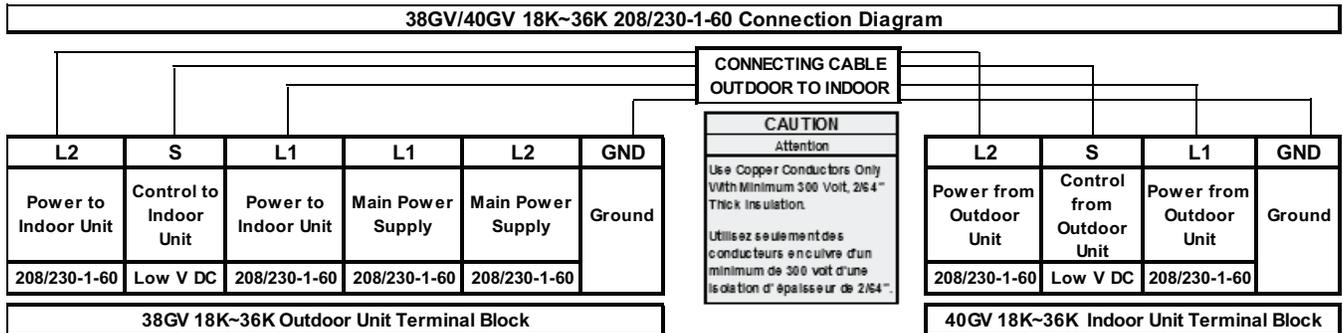
**NOTE:** Polarity of power wires must match original connection on outdoor unit.
